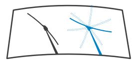
Raise the wiper arm away from the windshield and flip the rubber blade so it faces up.
