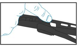
5. Push down firmly on the tab to lock the new wiper blade in place.
