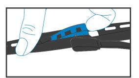
2. Disengage the lock by pulling the tab up.
