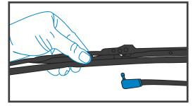
3. Pull the pin out of the hole on the side of the old wiper blade.
