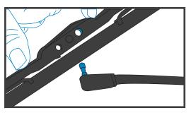
4. Pull the tab up slightly, and then insert the wiper arm pin into the new wiper blade.
