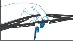
4. Insert the hook into the new wiper blade.
