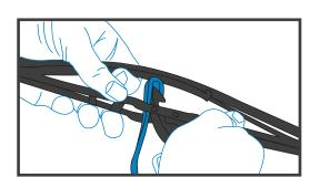
3. Lift up and remove the hook from the old wiper blade.
